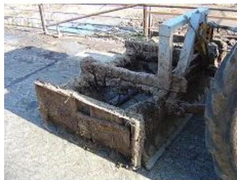
Fig 3:A box scraper will scrape cleanly, especially along kerbs, but will also save labour time making it an extremely cost effective investment.
